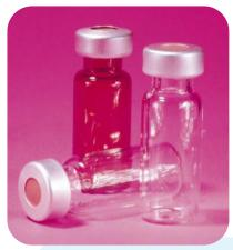
"Nitrogen purged" or dry vials are used for low-level water determination. These vials are necessary when an analysis requires that a vial be essentially water free to minimize interferences. Typical applications are in the analysis of residues and agricultural products.
